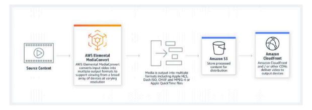
MediaConvert is used for video transcoding. The source video is converted into two different kinds of output: MP4 and HLS (allowing users access to multiple resolutions they can switch between during playback). MediaConvert also generates thumbnails by extracting multiple evenly distributed frames in the video to provide a preview capability.
